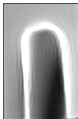
Titanium Rod Ø5mm in MRI field: demonstrates massive artifacts
